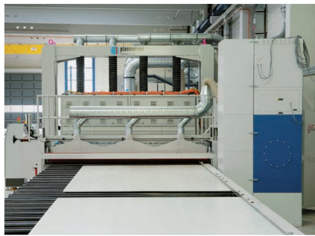
Figure 3 > Before priming with filler and painting, the large PP sandwich panels at MonoPan are pretreated with atmospheric pressure in a fully automatic process lasting just 20 to 40 seconds.
