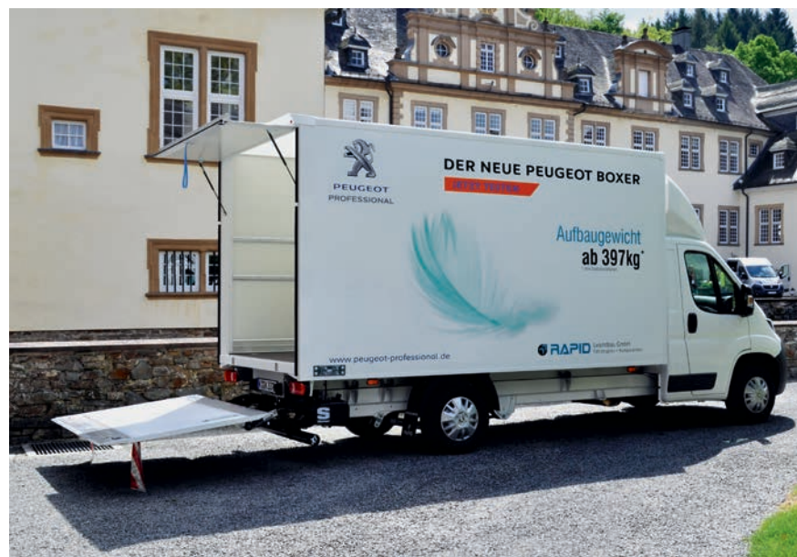
Figure 4 > The plasma-treated, pre-painted sandwich panels are used to construct low-weight box bodies for light trucks made by leading automotive manufacturers.
