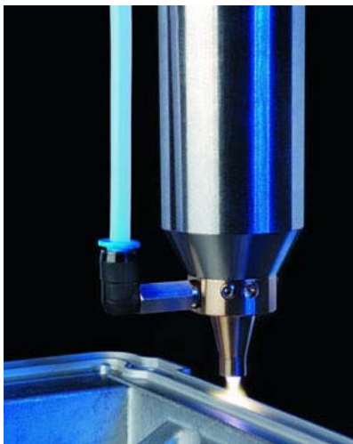
To provide a nanocoating on an electronics housing by the Openair PlasmaPlus process an organosilicon compound is added to the plasma Photo: Plasmacreat
