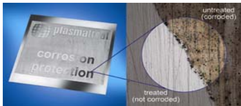
The photomicrograph shows that the region protected by the PlasmaPlus layer exhibits no sign of corrosion even after 96 h exposure to the salt spray test Photo: Plasmatrete
