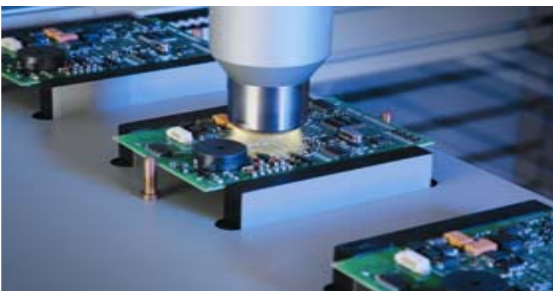
Photo Plasmamatreat To ensure long-term adhesion of the hotmelt, ultrafine cleaning and activation of the printed circuit board is carried out before sealing.
