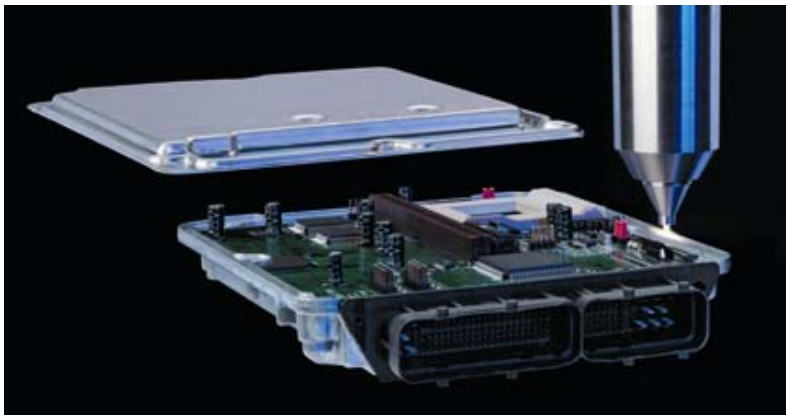
Photo: Plasmamatreat Pretreatment and activation of the housing surfaces with atmospheric-pressure plasma – before application of adhesive – brings about optimum leak-proofing of the packaging of the electronics.
